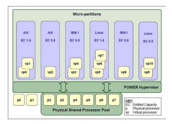
The IBM i partition configured to use virtual processor capacity indicated in the graphic above as vp8 is currently shut down, but the administrator needs to reserve the shared processor pool capacity for use with the IBM i partition once it starts up.
