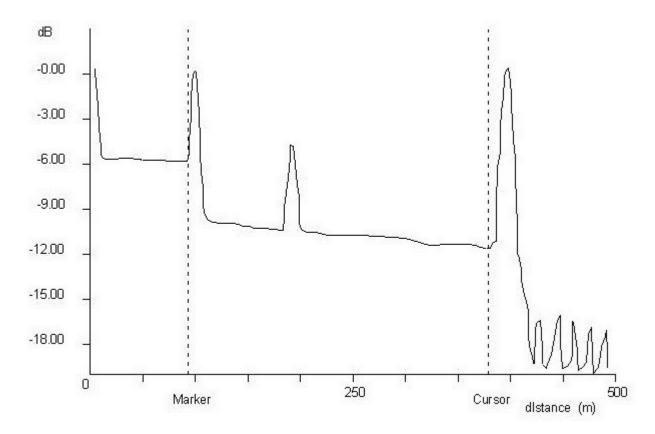
Which issue does the Optical Time Domain Reflectometer (OTDR) show?
