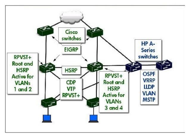
You are beginning the process of replacing Cisco switches at the distribution layer of your network with HP A-Series switches. Management has requested that network downtime must be kept to an absolute minimum. Your migration plan is to connect the A-Series switches in parallel with the distribution switches, as shown in the exhibit. For the A-Series switches to assume all routing functionality at the distribution layer, which configuration change should you complete first on the Cisco switches?
