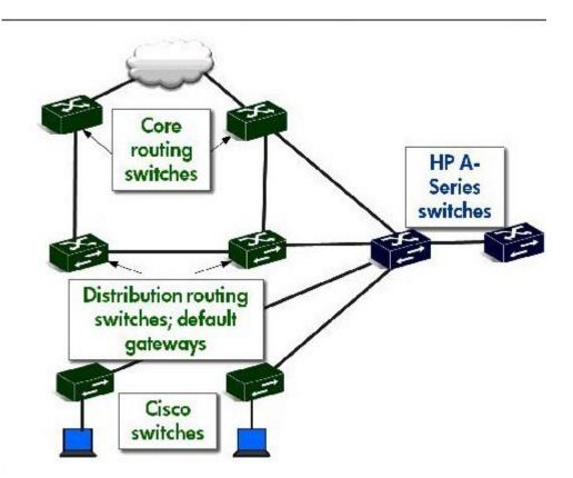
You are planning to replace Cisco distribution layer switches with HP A-Series switches, and you are selecting a general strategy for the migration process. The strategy you select is to connect the new switches in parallel to the existing network. You will move the edge switch connections to the new distribution switches during the migration, as shown in the exhibit What is a disadvantage of this strategy?
