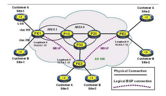
A provider of MPLS services configures MPLS Layer-3 VPN services for two customers. Each customer has three branch offices that will be interconnected by MPLS Layer-3 VPNs. The following are address blocks chosen by the customers for each site as shown in the chart:
