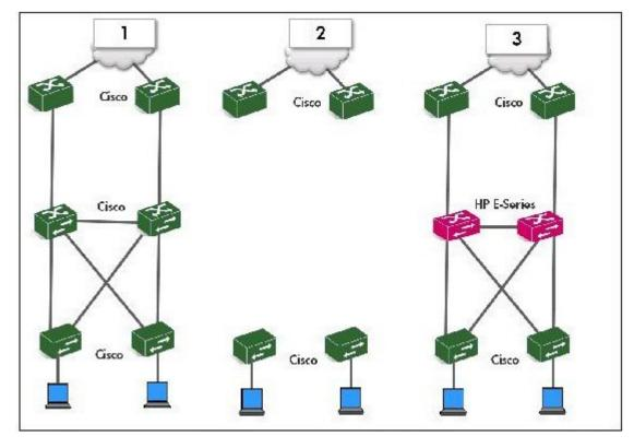
The exhibit displays the basic steps in one migration process for replacing Cisco distribution layer switches with HP E-Series switches. For which of these customers would this method be acceptable?
