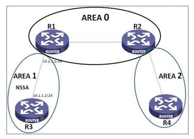
You have been asked to troubleshoot a problem in a multi-area OSPF network. Users connected to R3 are not able to access any destinations outside of Area 1. The Area 1 configurations for the R1 and R3 routers are shown below. Which configuration change should be made to correct this problem?
