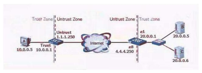
If A initiates a Web browsing session with B, and the Trust interface of the 5XT is in NAT mode, what could be the source address/port of the packet arriving at host B?
