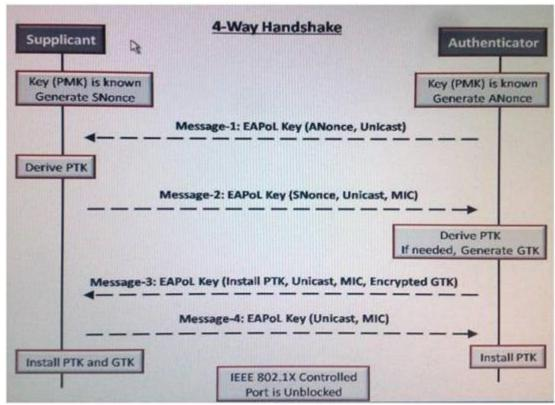
In this diagram illustrating an example of IEEE 802.11standard's4-Way handshake what is the purpose of ANonce and Snonce?
