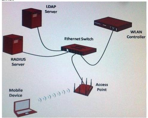
Given: The network in this diagram implements an 802.1X/EAP-based wireless security solution. What device functions as EAP authenticator?
