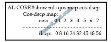
During deployment, a network engineer notices that voice traffic is not being tagged correctly as it traverses the network. Which COS to DSCP map must be modified to ensure that voice traffic is treated properly?
