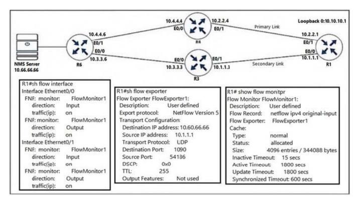
An engineer configured NetFlow on R1, but the flows do not reach the NMS server from R1. Which configuration resolves this Issue?
