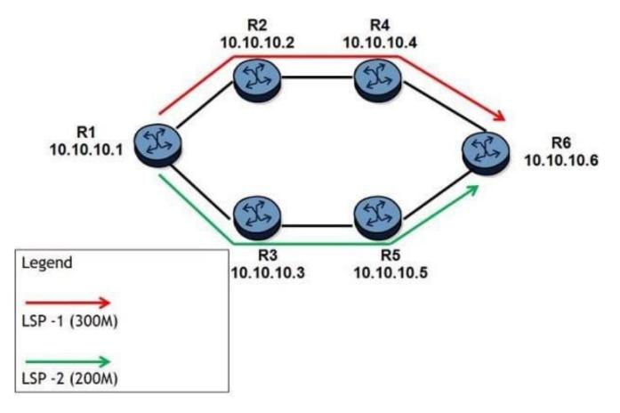
All links have 1 Gbps unreserved bandwidth initially and all LSPs have the least-fill feature enabled. After the two LSPs have been signaled as shown, two additional LSPs are configured.
