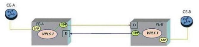
The SAP on PE-A has been configured with dot1q encapsulation. The SAP on PE-B has been configured with qinq encapsulation. CE-A sends frames with a single tag of 100. The VLAN tag from CE-A must be passed transparently. CE-B is expecting a frame with a top tag of 200 and bottom tag of 100. Which of the following is the correct SAP id for PE-B?
