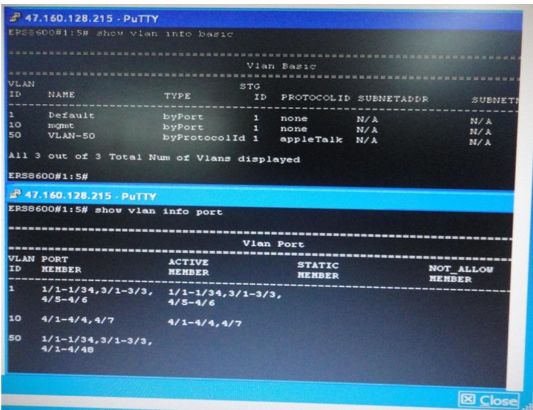
After checking the VLAN configuration using the show vlan info basic and the show vlan info port commands, there are no ACTIVE MEMBER ports for VLM4-50.
