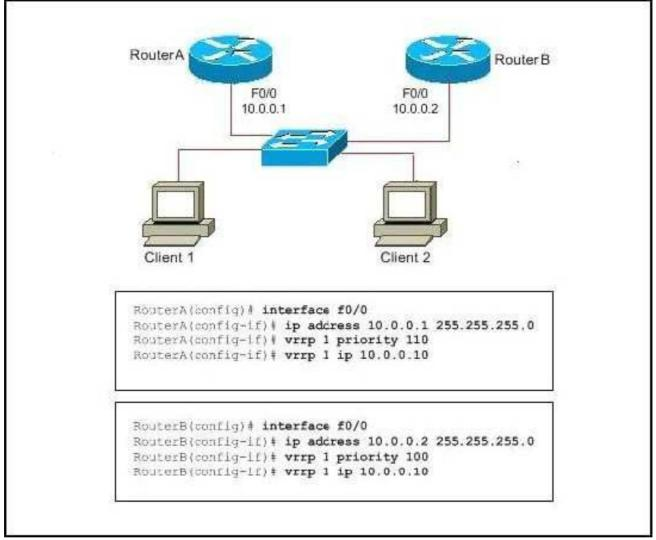
A. Router A is the master virtual router, and Router B is the backup virtual router. When Router A fails, Router B will become the master virtual router. When Router A recovers, Router B will maintain the role of master virtual router.
