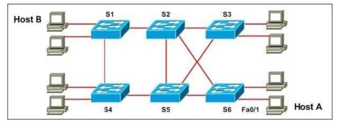
A. Fifty percent of the traffic will successfully reach Host B, and fifty percent will dead-end at switch S3 because of a partial spanning-tree loop.
