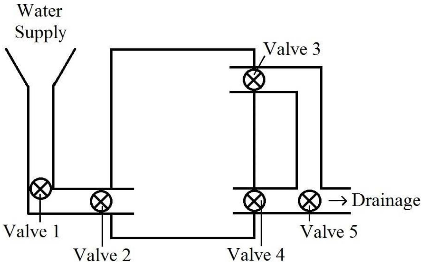
In the figure above, assume the valves are all closed. Which valves need to be open to fill the tank entirely?
