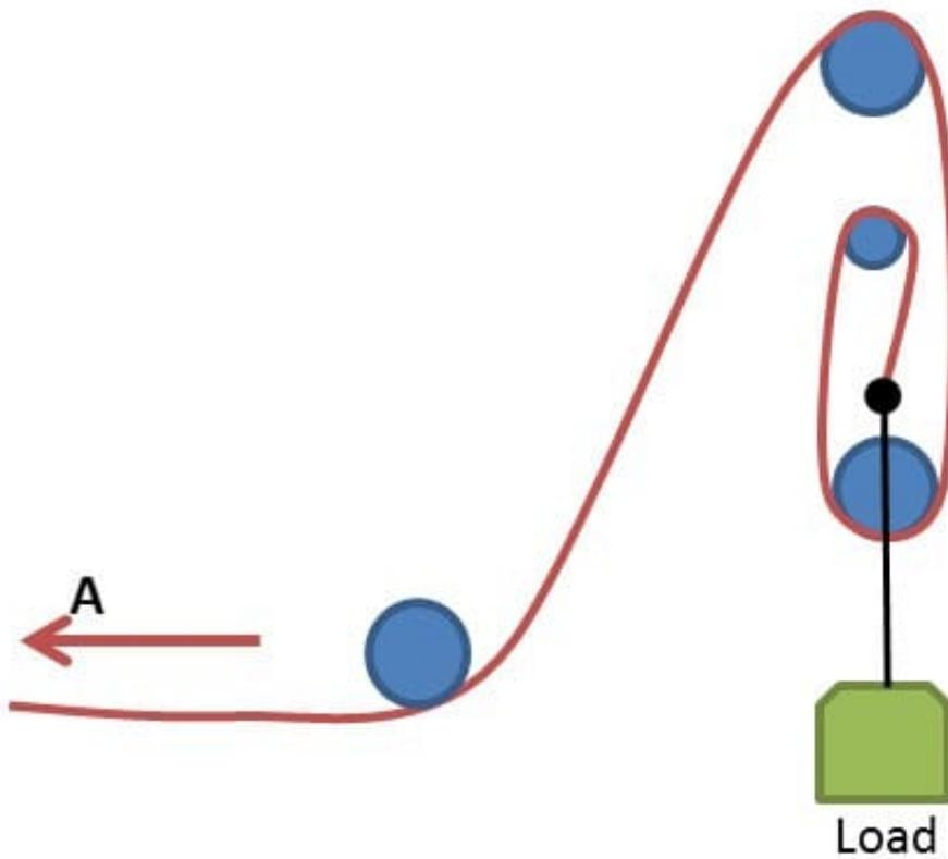
Pulling on the rope at point A will lift the load.
