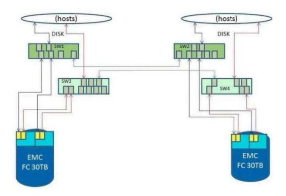
The exhibit illustrates the customer's environment. The IT infrastructure is located in two buildings less than six miles (10 KM) apart. The customer follows a two vendor policy. IBM is invited to advise the customer. The equipment is 18 months old and will not be removed for another 18 months. The customer needs another 30 TB on both sides and the growth will be 100% per year.
