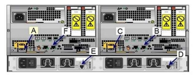
A service engineer needs to collect logs from SP B due to an unscheduled reboot. Which letter indicates the location where the service engineer would connect to SP B?
