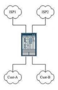
In the exhibit, Customer A and Customer B connect to the same SRX Series device. ISP1 and ISP2 are also directly connected to the SRX device. Customer A's traffic must use ISP1, and Customer B's traffic must use ISP2.
