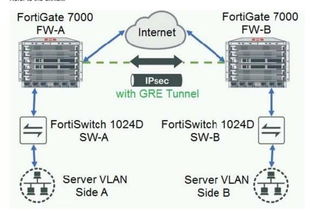
You have two data centers with a FortiGate 7000-series chassis connected by VPN. All traffic flows over an established generic routing encapsulation (GRE) tunnel between them. You are troubleshooting traffic that is traversing between Server VLAN A and Server VLAN B. The performance is lower than expected and you notice all traffic is only going through the FPM in slot 3 while nothing through the FPM in slot 4.
