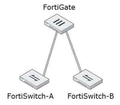
An administrator wants to implement a multi-chassis link aggregation (MCLAG) solution using two FortiSwitch 448D devices and one FortiGate 3700D. As described in the network topology shown in the exhibit, two links are already connected from the FortiGate to each FortiSwitch.
